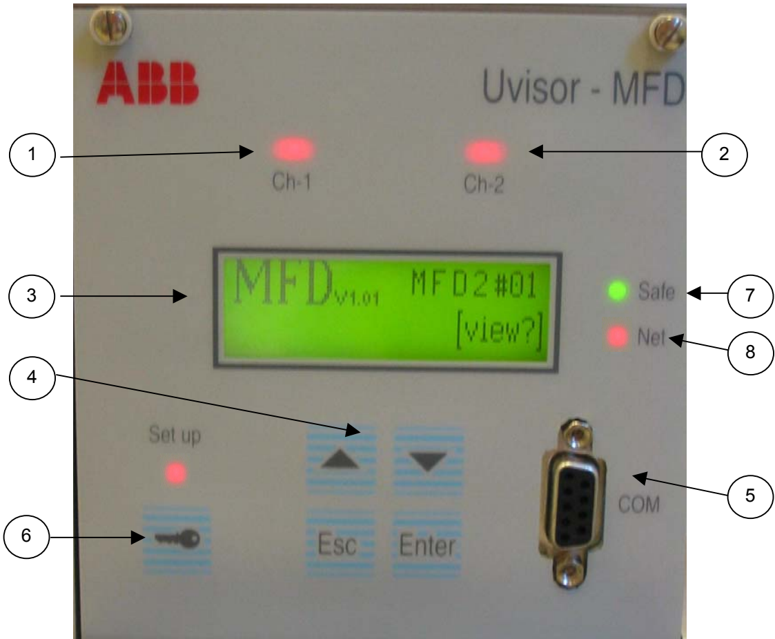
Figure 2. MFD Front panel
